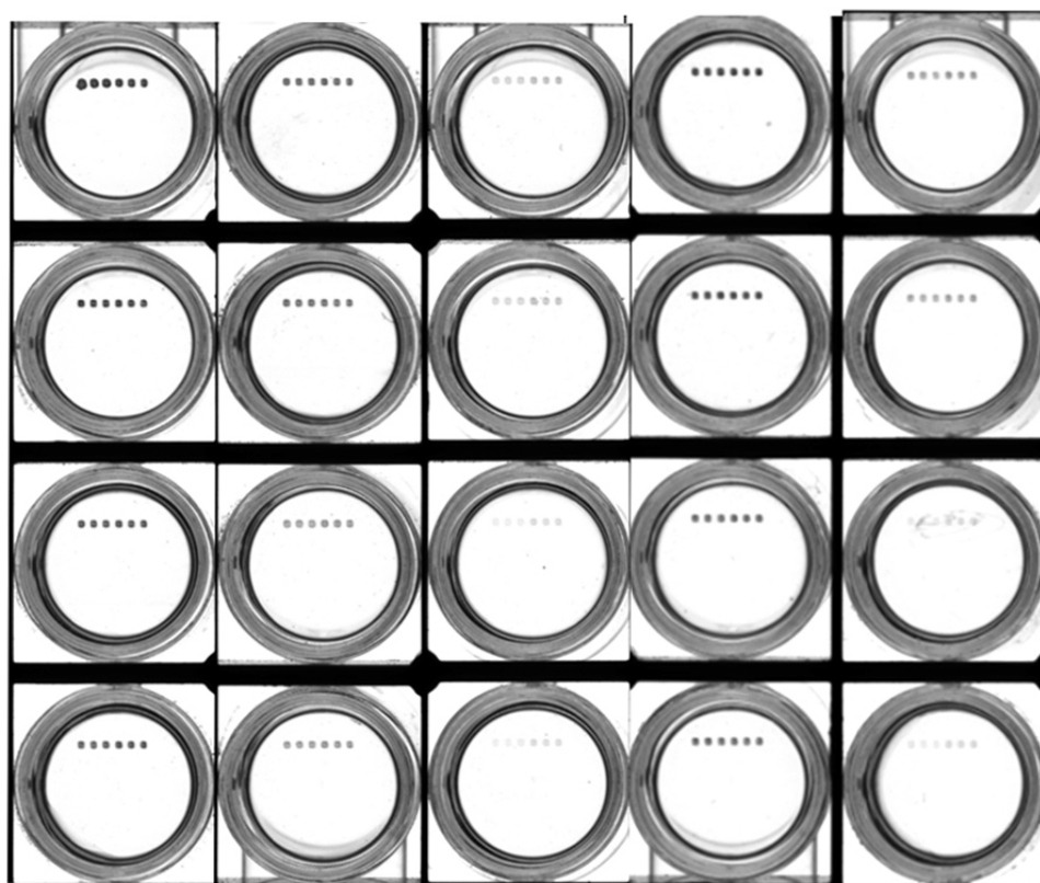
Figure 5: Picture of results of Ofloxacin and lomefloxacin detected by Visualized Microarray. From top to bottom, left to right was different concentrations of ofloxacin and lomefloxacin (0, 0.05 ppb, 0.2 ppb, 0.8 ppb, 3.2 ppb, 12.8 ppb), and milk sample which spiked different concentrations (0, 1 ppb, 10 ppb, 100 ppb). Samples were repeated 2 wells
