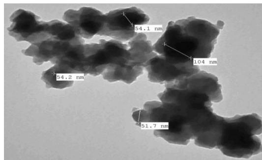
**Figure 18:** The transmission electron microscope of poly o-chloroaniline (POCIA)
