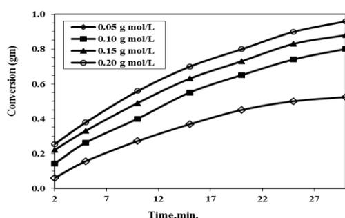
Figure (8): Conversion -time curves for the aqueous oxidative chemical polymerization of (OCIA).
