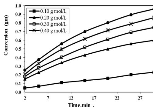
**Figure (6):** Conversion -time curves showing the effect of HCl concentration on the aqueous oxidative polymerization of (OCIA)
