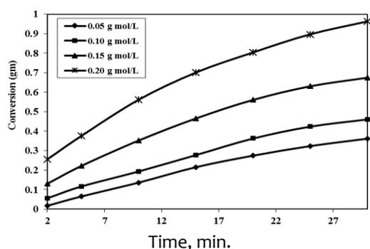
**Figure 4:** Conversion - time curve of the effect of potassium dichromate concentration on the polymerization of OCIA.
