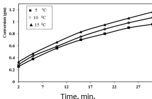
Figure 10: Conversion -time curves for the effect of temperature on the aqueous oxidative chemical polymerization of (OCIA).
