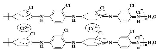
**Scheme (1).** Structure of the prepared poly o-chloroaniline.
