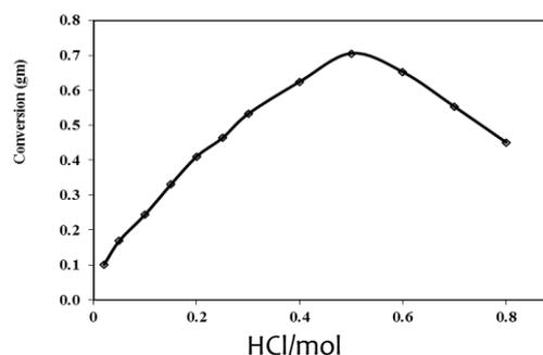
Figure 2: Effect of HCl concentrations on the aqueous oxidative chemical polymerization of (OCIA).
