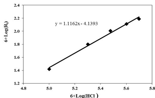
**Figure (7):** Double logarithmic plot of the initial rate and HCl concentration on the oxidative chemical polymerization of (OCIA).
