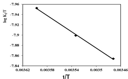
**Figure 12:** The relation between  $\log K_2/T$  and  $1/T$  for oxidative chemical polymerization of (OCIA)
