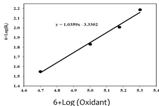
**Figure 5:** Double logarithmic plot of the initial rate and oxidant concentration for polymerization of (OCIA).
