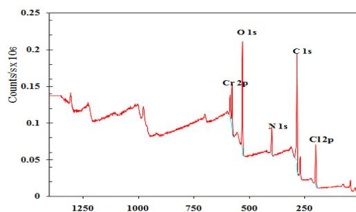
**Figure 13:** X-Ray Photoelectron Spectroscopy (XPS) survey elemental composition of (POCIA).
