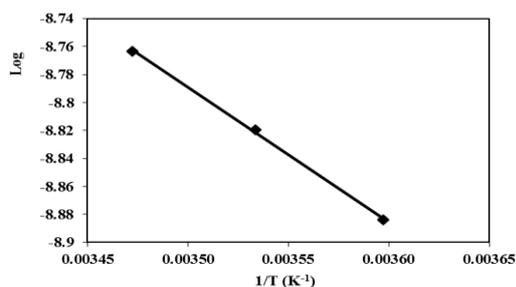
Figure (11):The relation between the logarithm of initial rate and ( $1/T$ ) for aqueous oxidative polymerization of (OCIA)
