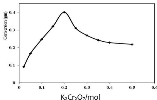
Figure 1: Effect of  $\text{K}_2\text{Cr}_2\text{O}_7$  concentration on the aqueous oxidative chemical polymerization of (OCIA).
