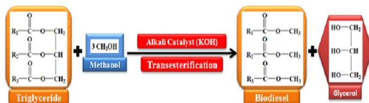
Figure 1: experimental conditions for converting triglyceride to biodiesel (Transesterification)
