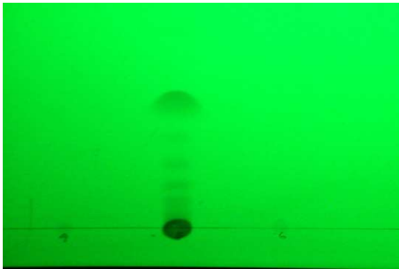
Fig.2: TLC plate observed at 240 nm
