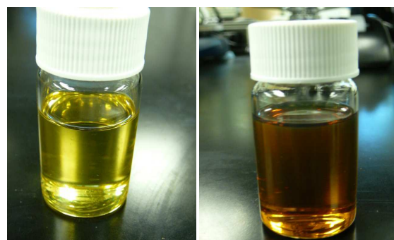
Figure.4: PP and PS waste plastic mixture to fuel with activated carbon (Yellow color) and PP and PS waste plastic to fuel without activated carbon (Brown color)
