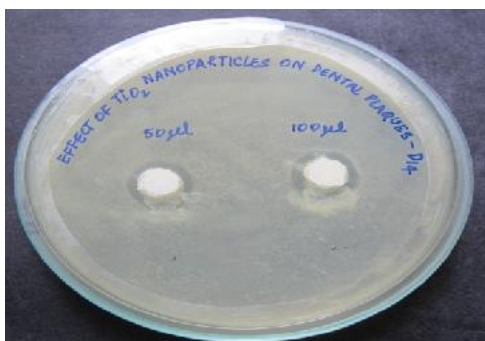
Fig. 2.2: Analysis of the Antimicrobial activity of TiO 2 Nano Particle on D14 sample showing that TiO 2 is inhibiting the growth of the organism
